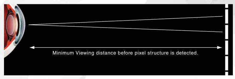
To avoid eye strain, it is recommended that the closest operators to the display wall should not be able to see the pixel structure of the displays. Optimum Viewing Distance is the distance before pixel structure is detected.
